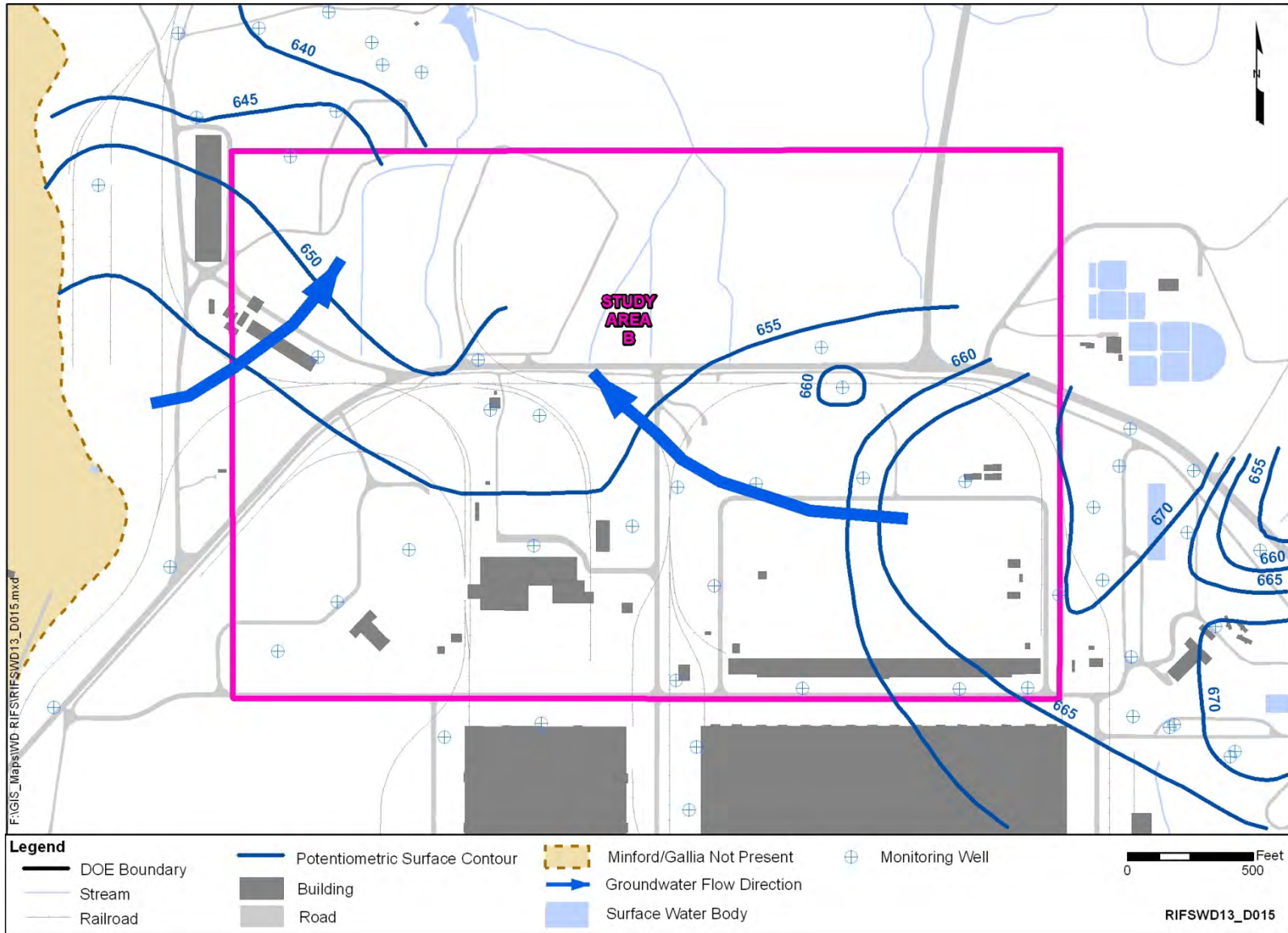
Figure D.15. Potentiometric Map of the Minford/Gallia in Study Area B at PORTS
