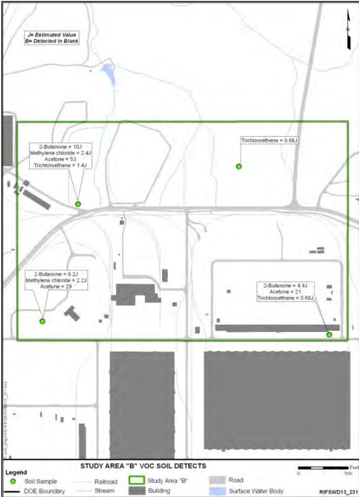
Figure 2.32. VOCs Detected in Soils at Study Area B
