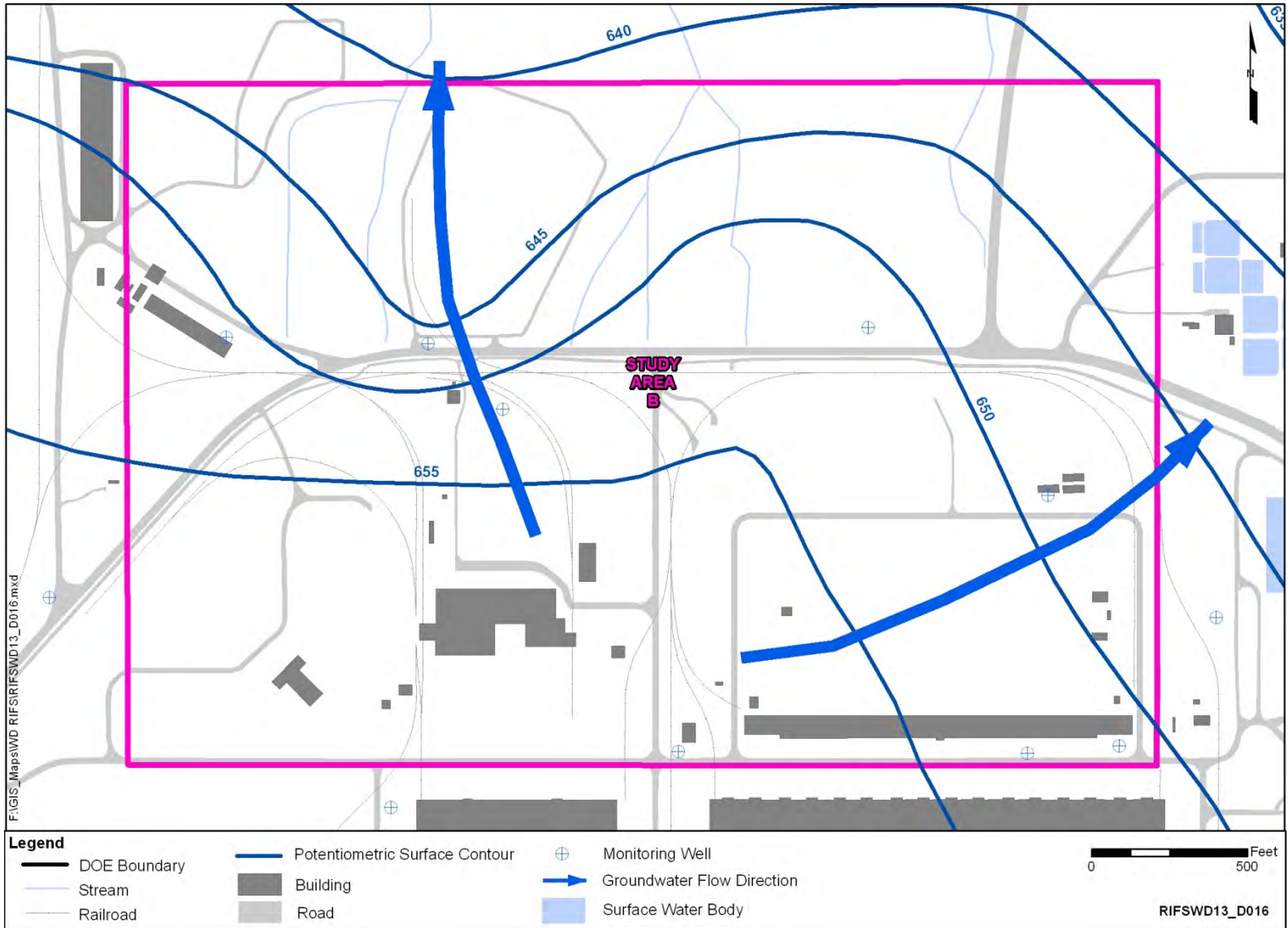
Figure D.16. Potentiometric Map of the Berea Sandstone in Study Area B at PORTS
